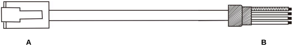
Figure 4.9 Schematic diagram of communication cable between servo driver and PLC
